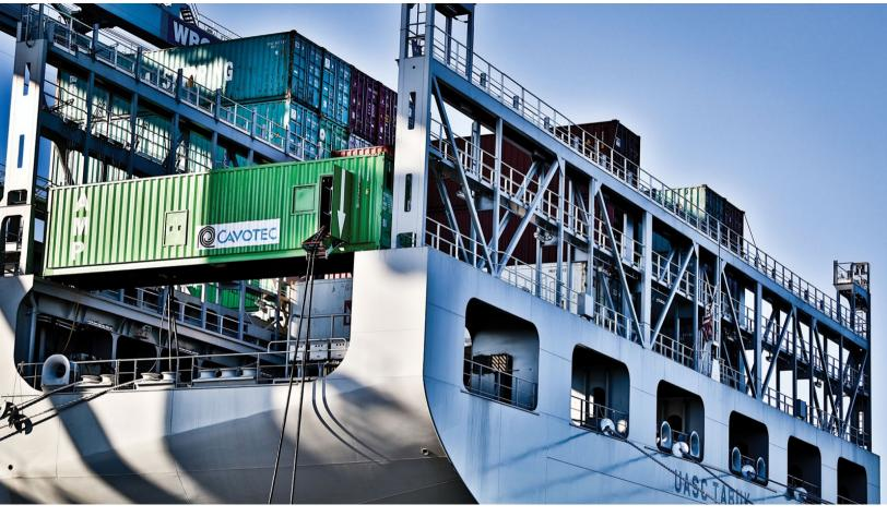
Cavotec PowerFit is a complete containerised solution and includes all equipment for a high voltage shore connection.
