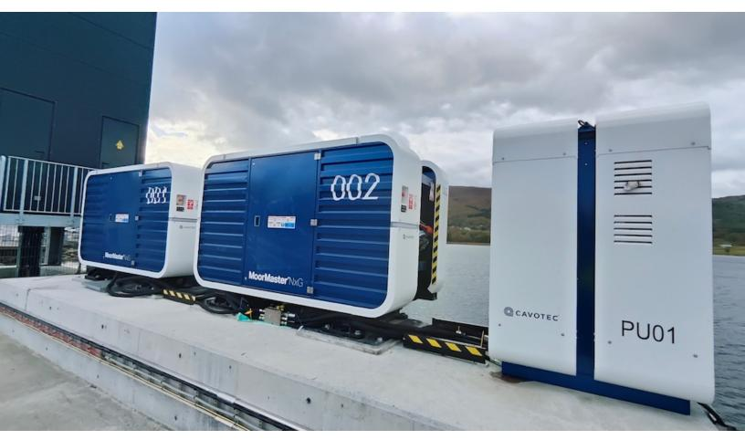
MoorMaster NxG will fully automate vessel mooring and keep the electric ferries precisely positioned, enabling fast shore connection and reliable charging at the ports of Odden and Aarhus..
