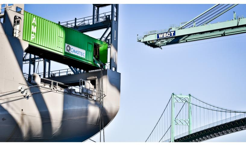
Cavotec PowerFit containerised shore power system enables retrofitting process to take place while vessels are sailing.
