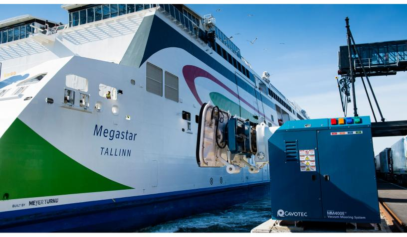
A new port efficiency tool developed by DNV GL Maritime Advisory indicates that the Port of Helsinki's use of a MoorMaster™ automated mooring system reduces vessel fuel consumption by up to 2,800 tonnes every year.
