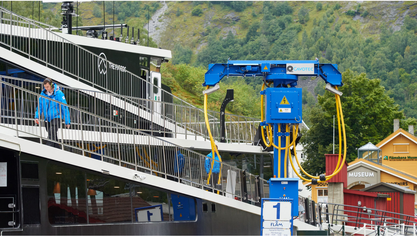
All set: a shore power dispenser unit charging the Vision of the Fjords at the Flåm berth in Norway.
