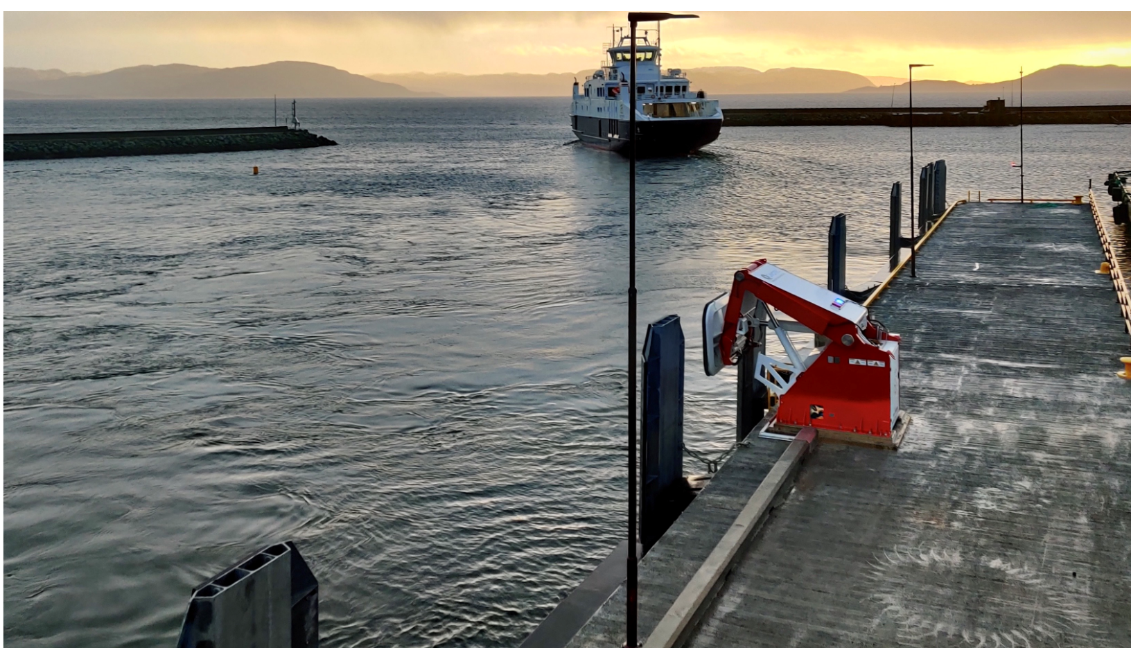
A MoorMaster™ vacuum mooring systems at a ferry application in Norway.
