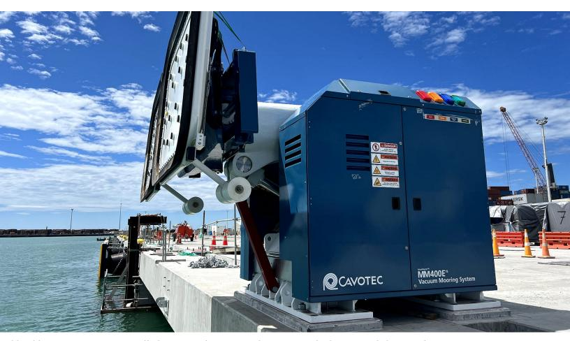
MoorMaster uses remote controlled automated vacuum pads to moor and release vessels in seconds.
