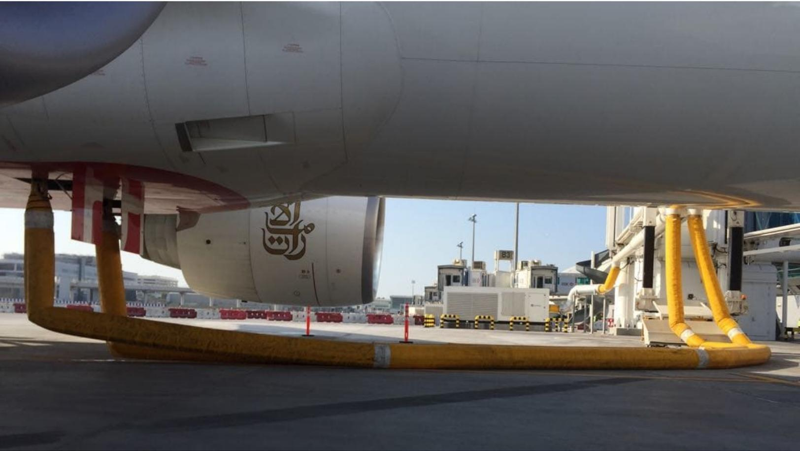
Cavotec PCA systems ensure aircraft are cooled quickly and efficiently.
