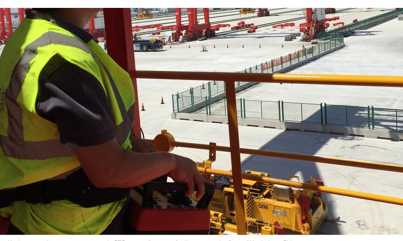
Under control: an operator controls STS cranes from a safe distance at the Port of Yanhshan, China.
