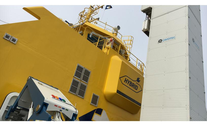
A MoorMaster™ unit moors the Electra hybrid ferry, as the Automatic Plug-in System readies to charge the vessel.
