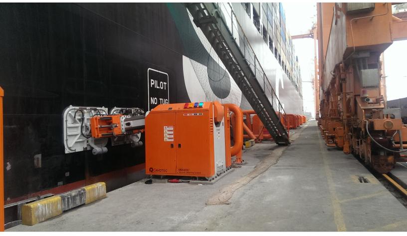
Safe and sound: MoorMaster automated mooring units hold a container vessel in position at Salalah.
