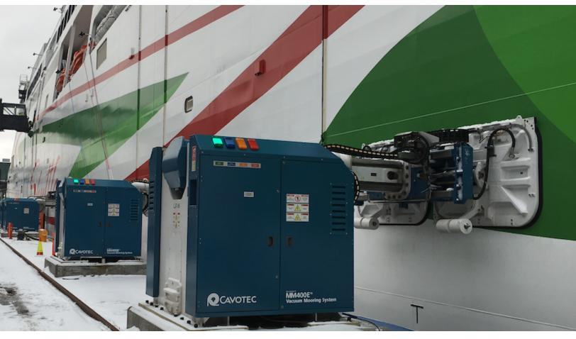
MoorMaster™ units hold the 212m Tallink Megastar passenger ferry in perfect position at Port of Helsinki's LI7 berth.
